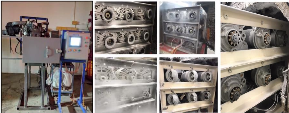
Vibration, Heat, Cold, Sand, Dust, and Salt Spray Endurance Testing
