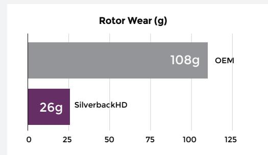
SilverbackHD pads yield up to 75% less rotor wear than leading OEM brands in FMVSS 121 testing
