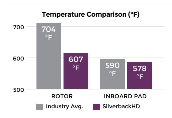
SilverbackHD pads keep the rotor temp. around 100 degrees cooler, resulting in longer service life.
