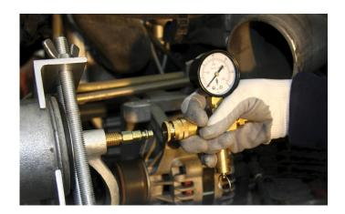
Charge air cooler testing
